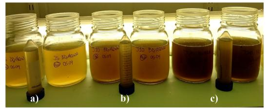
Fig. 4. Phase III, color and turbidity of BD/ACE blends at t0, prior to inoculation; a) 5:95 BD:ACE, b) 10:90 BD:ACE, c) 20:80 BD:ACE.
