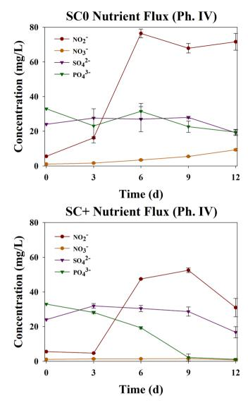
**Fig. 13.** Phase IV nutrient flux  $(NO_2^-, NO_3^-, SO_4^{-2-})$  and  $PO_4^{-3-})$  under each experimental condition; a) without scaffold, b) with scaffold.
